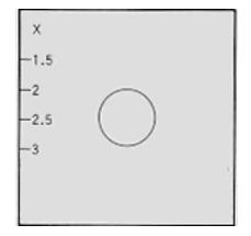
The figures on the focusing screen left side indicate the exposure factor. Compensate in the exposure after reading the figure indicated by the pointer while focusing. For instance, assuming that the correct exposure value measured by an exposure meter is 1/125 sec. at f/11,
